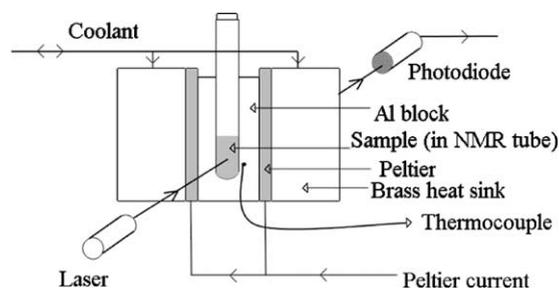
Fig. 2. A schematic of ALTA4, showing the cooling system and the optical sensing of solidification of the sample. Note that the thermocouple is close to, but outside the sample.
